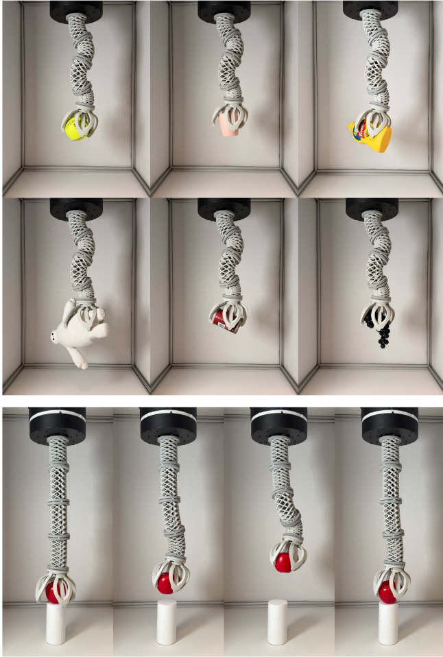
Fig. 10: Object grasping. Top: The gripper successfully adapts to objects of various shapes, sizes, and stiffnesses. Bottom: Sequential images showing the robot picking up an apple from a pedestal and placing it back down.
