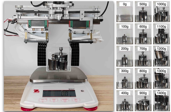
Fig. 7: Experimental setup for sensing different weights. (Left) For each of 7 pre-defined grasp strengths, the gripper makes 3 attempts to grasp a box filled with weights. A digital scale confirms a successful lift-off. (Right) The experiment is repeated with 15 weights from 0 to 1400 g.
